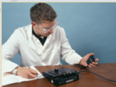
Figure 7.1.3 At intervals of time measured using a stopwatch the digital colorimeter reading is recorded.
