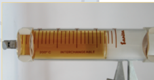
Figure 8.2.9 A gas syringe with movable piston containing an equilibrium mixture of \text{NO}_2 and \text{N}_2\text{O}_4 .
