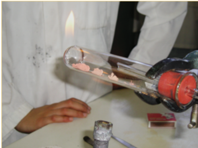
Figure 10.1.2 Copper oxide can be reduced to form copper in the laboratory.
