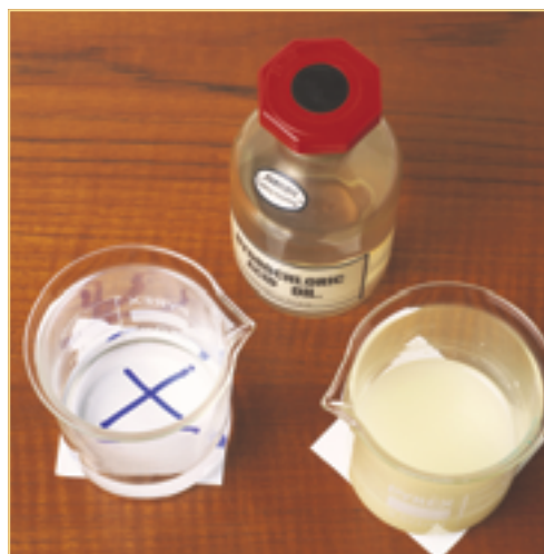
Figure 7.1.6 The reaction between sodium thiosulfate and hydrochloric acid. When the amount of sulfur is great enough, the cross underneath the beaker cannot be seen.
