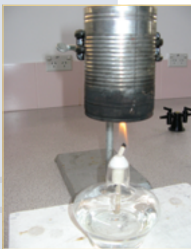
Figure 6.2.2 A simple apparatus for measuring the heat of combustion of a fuel.
